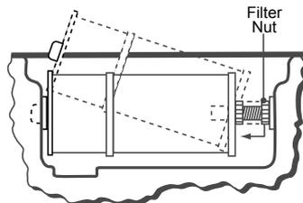
1. Install filter assembly, then tighten filter nut so it just touches filter face. **DO NOT OVERTIGHTEN!**
