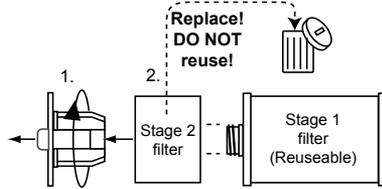
1. Rotate stage 2 retainer counterclockwise to release, then separate filter assembly.
