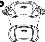
Gently pull outward on pillow to release mounting stud from receptacle on spa shell.
